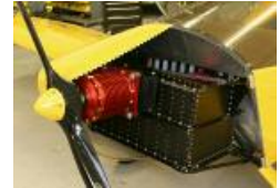
under the cowl of the Sonex e-plane - note battery boxes
