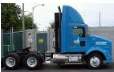
PG&E-CleanAir Transport 'Clean Air Machine,' a Kenworth tractor fitted for CNG or LNG operation, shown at Clean Energy's new Oakland fueling station
