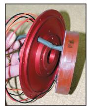
\_\_ 2. Attach the stator to the alternator mount plate using four (4) ACV-Z01-76 screws. Place a drop of Locktite 242 on each screw prior to installation.
