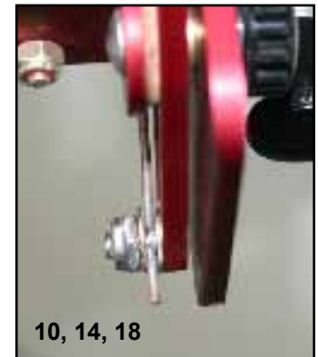
A set screw in the cable adjuster holds the cable housing in place.
