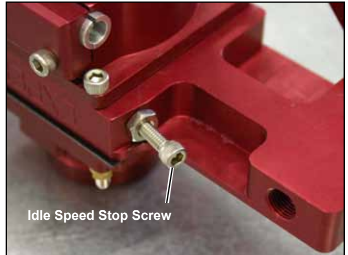
A 9/64" hex wrench is used to adjust the Idle Speed Stop Screw. The lock nut is tightened / loosened with an 11/32" open-end wrench.
