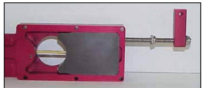
This cut-away view shows that at "Full Throttle", the throttle slide exposes the entire intake air passage.
