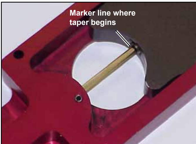
Screw the carrier into the Throttle Slide until the beginning of the taper is even with the edge of the slide, as shown in this cut-away.
