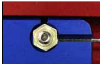
Install a socket set screw to lock the cable in place.
