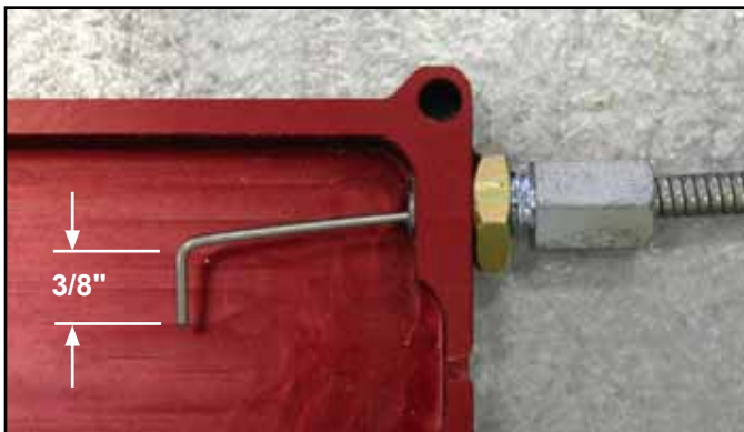
The solid wire is inserted through the cable adjuster and then bent 90 degrees.
