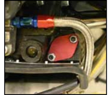
The oil temperature plate is not needed on all engine blocks. It is located on the front of the engine, below cylinder #2.
