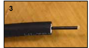
The boot included with the spark plug wires is slipped over the cut end of each wire.
