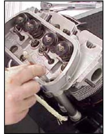
The pushrod length tool is inserted in a pushrod tube after removing the rocker shaft.
