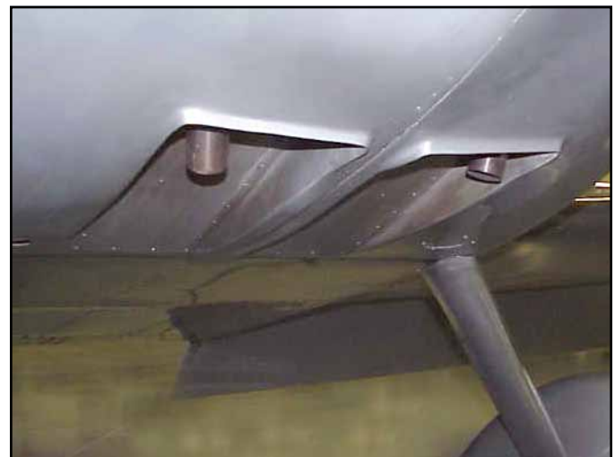
This view of a completed cowl clearly shows the air deflector lips which are added to the front of the exhaust cut-out. These lips create a low pressure area which draws the cooling air through the cowl. These lips are particularly important when the airplane is in a climb attitude. This aircraft is fitted with the old-style 4-piece exhaust.
