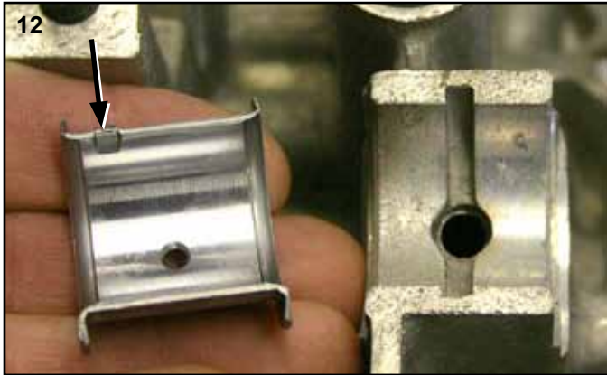
File the tab (arrow) off the flanged bearing with a fine file.
