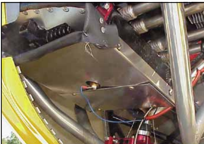
This airplane has had the oil cooler removed. Note the aluminum panel which closes off the oil cooler opening in the bottom of the shroud.
