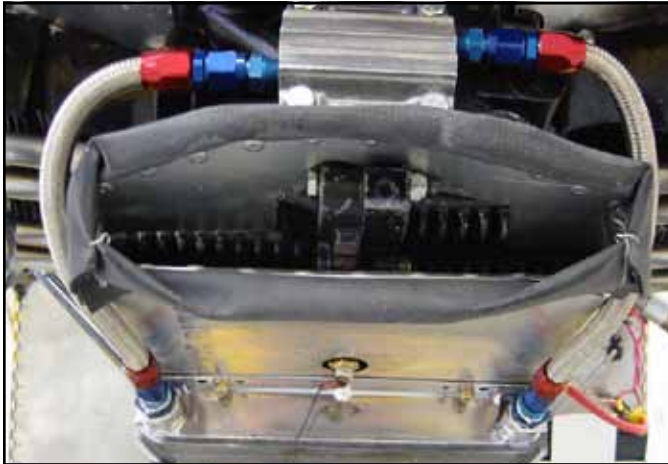
This photo shows the oil cooler lines attached to the oil pump.
