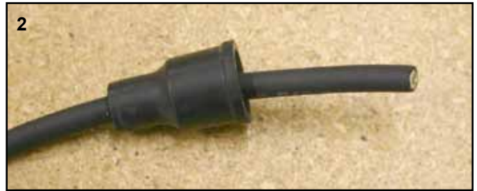
The boot included with the spark plug wires is slipped over the cut end of each wire.
