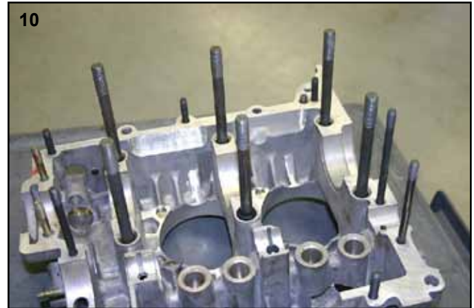
The Stud Seals slide over the 6 large studs in the right case half.
