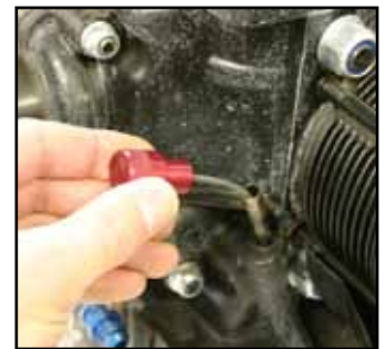
The oil temperature plate is not needed on all engine blocks. It is located on the front of the engine, below cylinder #2.
