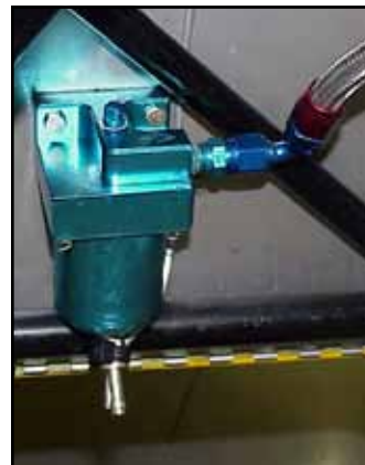
The fuel line at the gascolator can be fitted with either a 90° swivel fitting (left), or a straight fitting (right). The choice of which to use should be based on the best routing for the fuel line to avoid the exhaust pipes.
