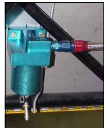
The fuel line at the gascolator can be fitted with either a 90° swivel fitting (left), or a straight fitting (right). The choice of which to use should be based on the best routing for the fuel line to avoid the exhaust pipes.
