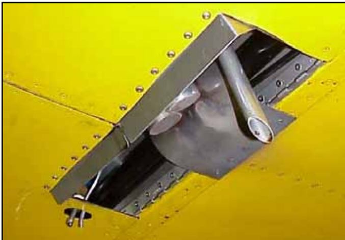
This photo shows the standard outlet for a 2-into-1 exhaust fitted to a cowl without pre-molded tunnels. If you are fitting a cowl with premolded exhaust tunnels, this opening must only be large enough to allow the exhaust pipes to exit. The small tube in this photo is the oil breather.
