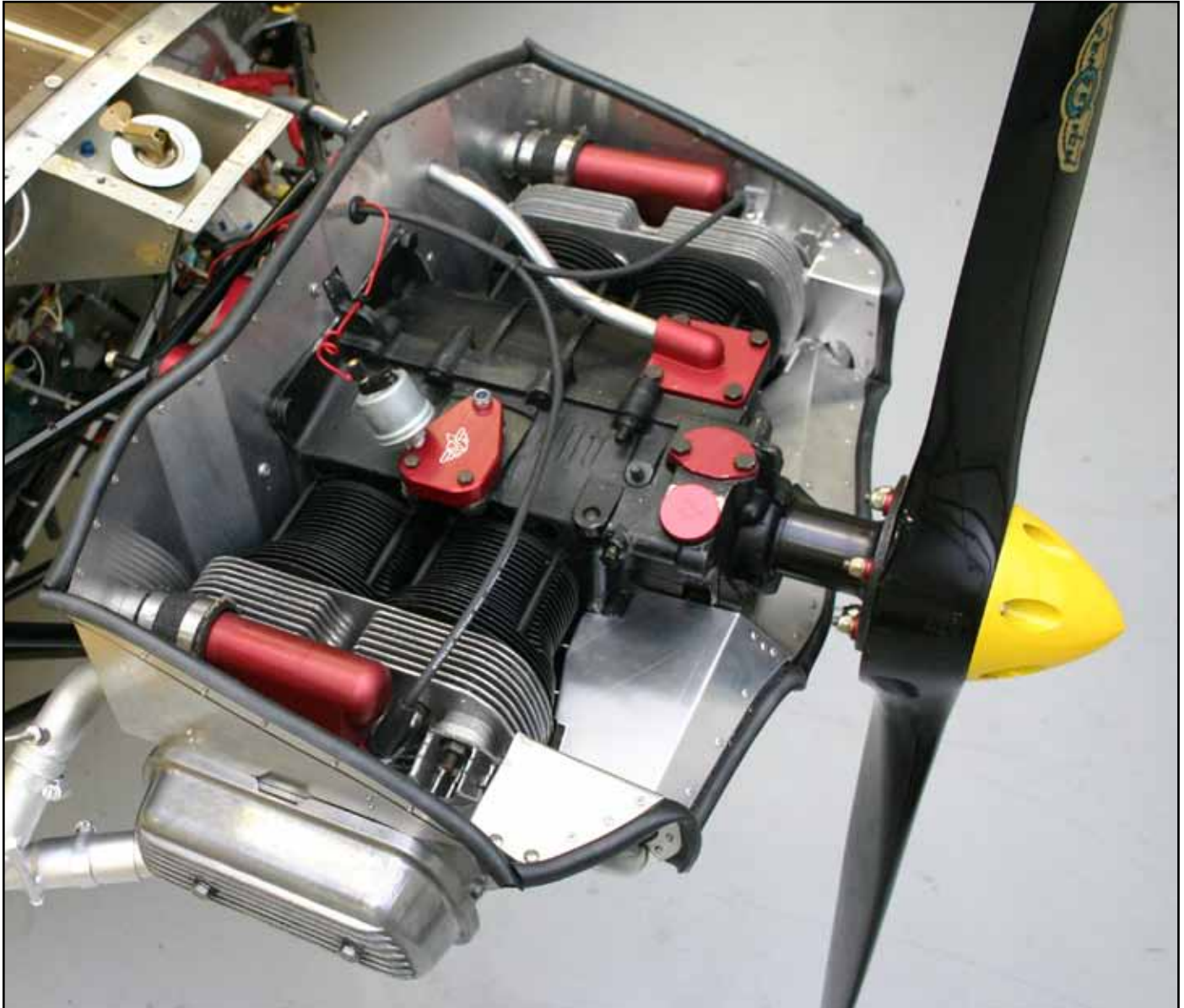
An AeroConversions' fence baffle fitted to a Sonex airframe. The installation shown here has a bottom-mounted oil cooler.
