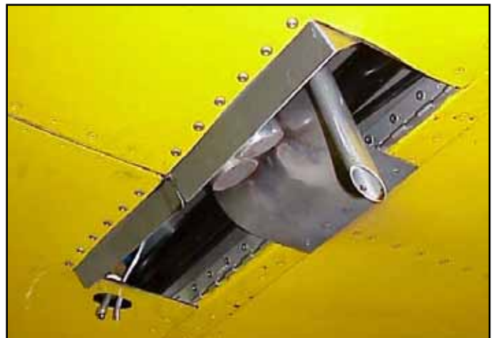
This photo shows the standard outlet for a 2-into-1 exhaust fitted to a cowl without pre-molded tunnels. The cut-out measures 4" x 12.5". No additional cowl outlets are needed for cooling air. The small tube in this photo is the oil breather.
