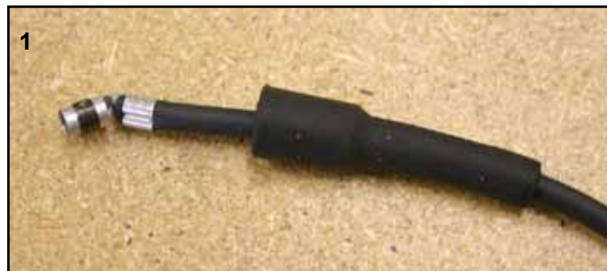
The crimped end of each plug wire is re-used - do not cut them off.
