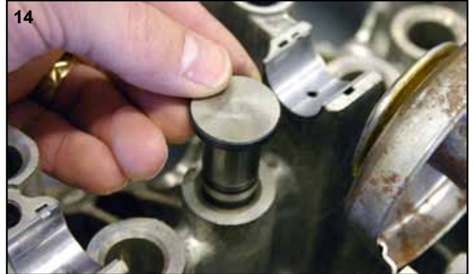
Test fit each valve lifter to assure smooth operation.
