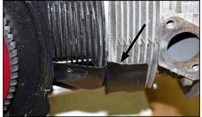
The super tin is installed under the cylinders and cylinder heads. Friction keeps it in place.
