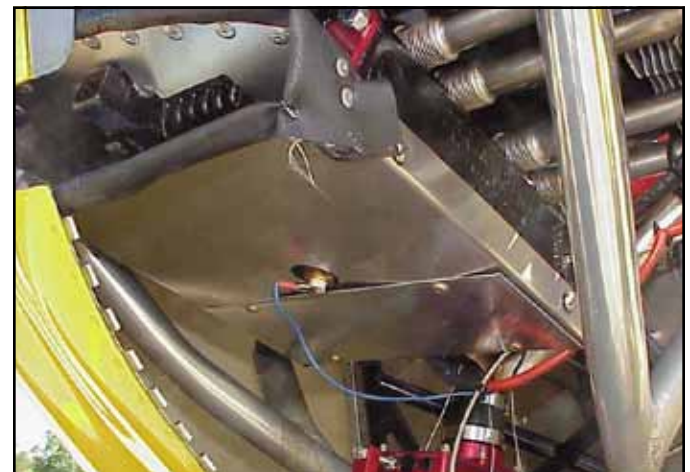
While the top photo gives approximate dimension for the location of the oil cooler inlet, fitting one cowl half and marking the exact location will ensure the correct fit for your airplane. Note that the oil cooler inlet is required even if no cooler is installed, as on this airplane.
