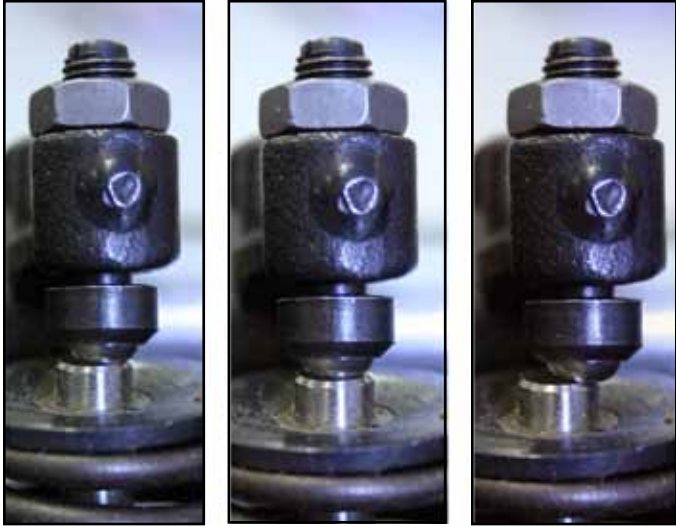
Correct - The flat of the swivel pad is off center from the valve stem but sits fully on the valve stem.
