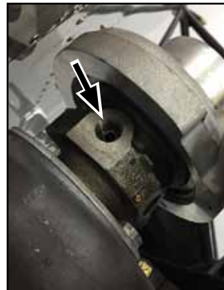
The oil supply port in the top of the turbo body and oil line fittings are shown here.
