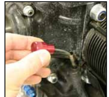
This oil temperature plate has been drilled for, and fitted with, an oil temperature probe. It is located on the front of the engine, below cylinder #2.
