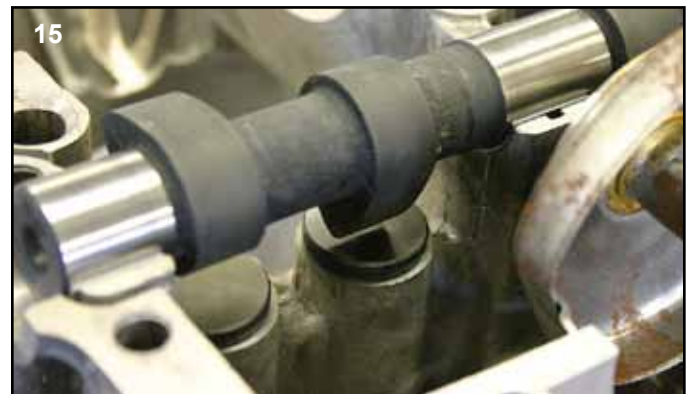
Test fit the camshaft to confirm there is clearance between the lobes of the camshaft and each lifter.
