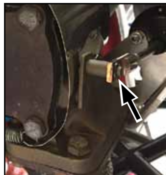
Secure the actuator arm with the snap ring provided.
