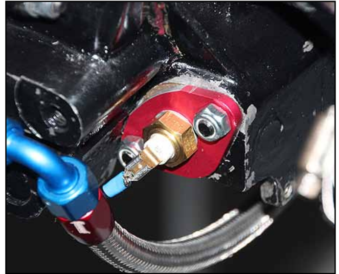
This oil temperature plate has been drilled for, and fitted with, an oil temperature probe. It is located on the front of the engine, below cylinder #2.
