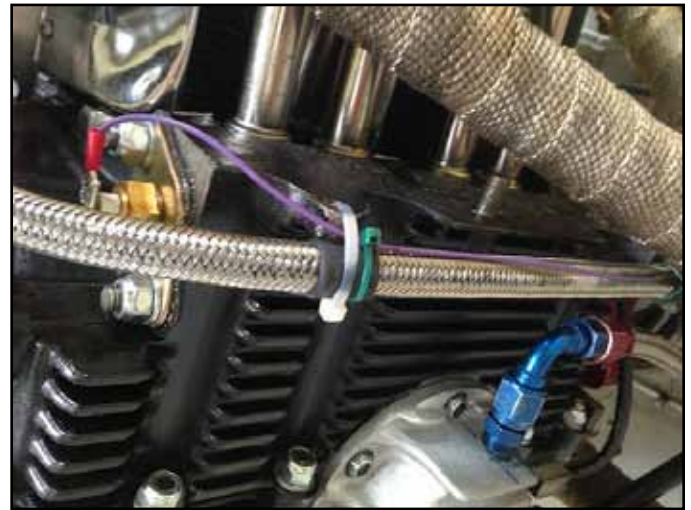
The oil line secured under the engine case. The oil line runs from the bottom of the Turbo Oil Drain Sump to the left port of the secondary oil pump (right photo).
