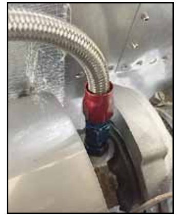
The oil supply port in the top of the turbo body and oil line fittings are shown here.
