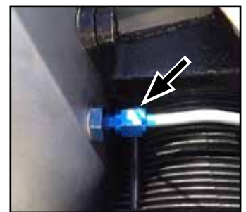
Looking down on the bulkhead fitting installed through the engine case flange and rear fence baffle.
