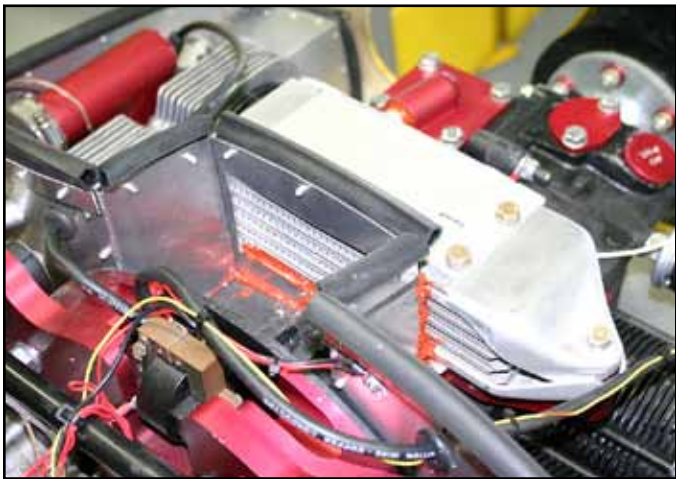
These two photos show the required baffling when a top-mounted oil cooler is installed.
