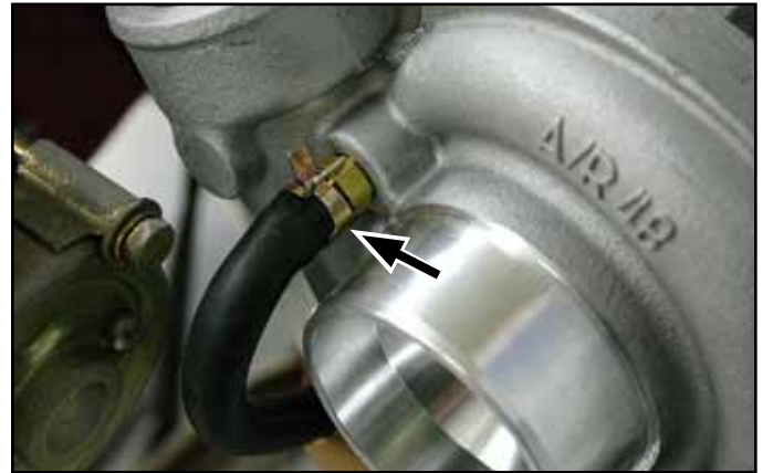
One end of the Actuator Air Balance line is secured to the nipple on the compressor portion of the turbo.
