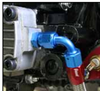
The oil drain sump is bolted (1) to the bottom of the turbo body. A 1/4 NPT to -06 hose fitting (2) is installed in the drain. The fitting may be straight or a 45-degree elbow.
