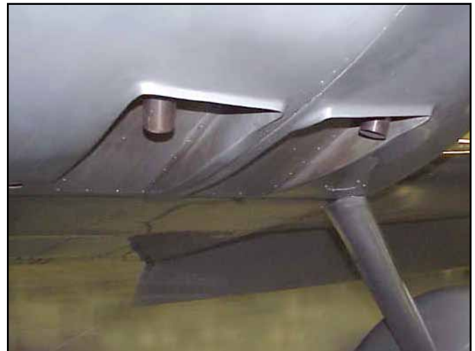
This view of a completed cowl clearly shows the air deflector lips which are added to the front of the hot air exit cut-out. These lips create a low pressure area which draws the cooling air through the cowl. These lips are particularly important when the airplane is in a climb attitude. This aircraft is fitted with a non-turbo exhaust. A turbo installation will require a hole be cut large enough to allow the turbo exhaust to exit the cowl without contacting the cowl (see photo next page).
