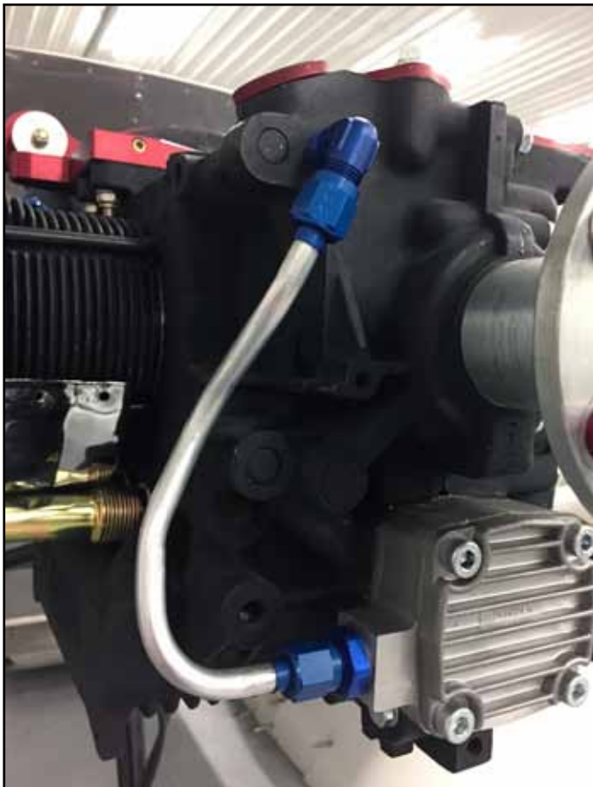
Oil line from the right port of the secondary oil pump to a hole tapped in the engine case approximately 1.5" below the oil fill cap.
