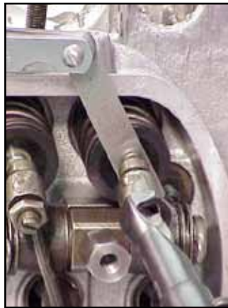
Here an exhaust valve is being adjusted to .014".
