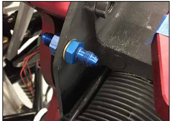
The bulkhead fitting installed through the engine case flange (fence baffle not shown in this photo).
