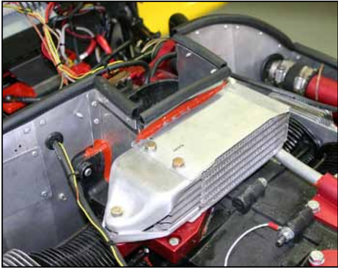
These two photos show the required baffling when a top-mounted oil cooler is installed.
