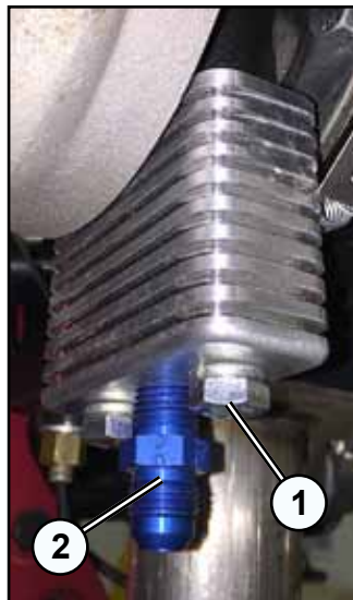
The oil drain sump is bolted (1) to the bottom of the turbo body. A 1/4 NPT to -06 hose fitting (2) is installed in the drain. The fitting may be straight or a 45-degree elbow.
