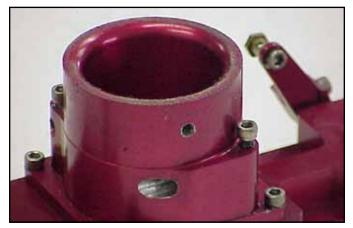
The intake bell drilled and tapped for the AN3-11A bolt provided with the air filter.
