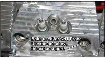
A cylinder head bolt above an exhaust port is used for accurate temperature indications. On the left side of the engine (as viewed from the flywheel end) it is the aft bolt, on the right the forward bolt.
