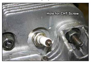
Drill the hole for the probe screw as close to the spark plug as possible. This photo shows the AeroConversions' suggested location for an AeroVee engine.
