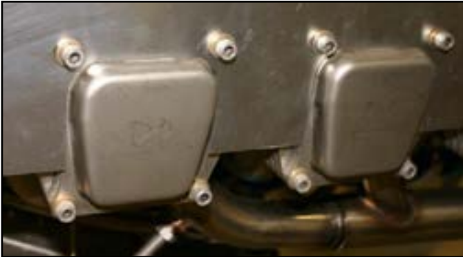
The upper valve cover screws secure the baffles in place.
