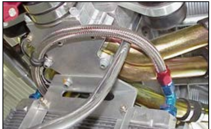
This photo, looking up at the bottom of the engine, shows the smooth bend the oil hose takes from the right side oil cooler port to the left side of the engine. While this is not an Aero Classic cooler installation, hose routing is the same.
