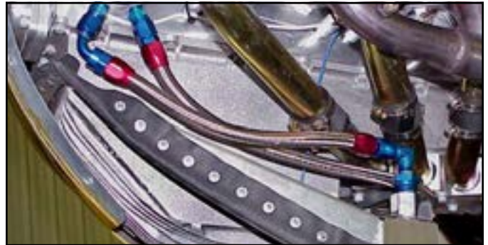
The installation of the oil hose on the left side of the engine is shown in this photo.
