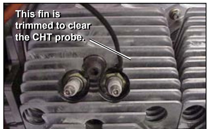
The fin above a spark plug with a CHT probe must be trimmed if you are installing CHT probes under the spark plugs. Always install CHT probes over the exhaust port side of a cylinder head. Probe installation is described in the wiring section of this manual.
