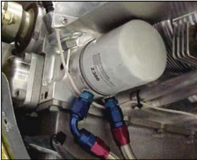
The barbed fittings are removed from the Jabiru-provided oil cooler adapter and replaced with threaded hose fittings.
