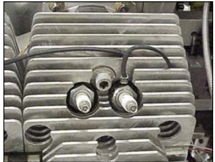
A CHT probe installed on the left-rear cylinder. The CHT wires are routed between the cylinder fins to the rear cylinder, where they turn down and exit below the cooling shroud.
