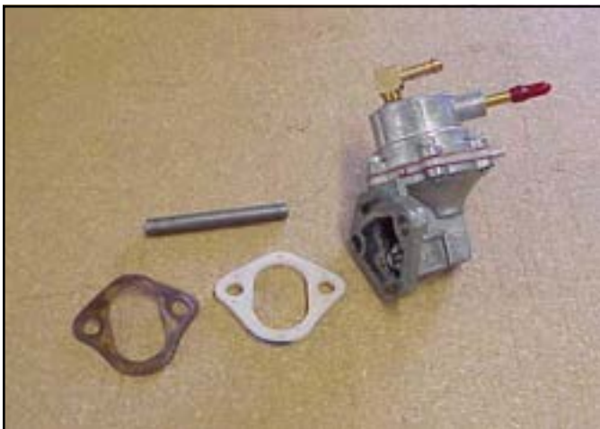
The fuel pump and related parts are removed from the engine.
