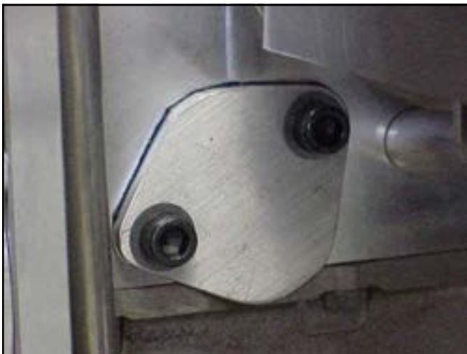
The fuel pump block-off plate is installed in place of the fuel pump.
