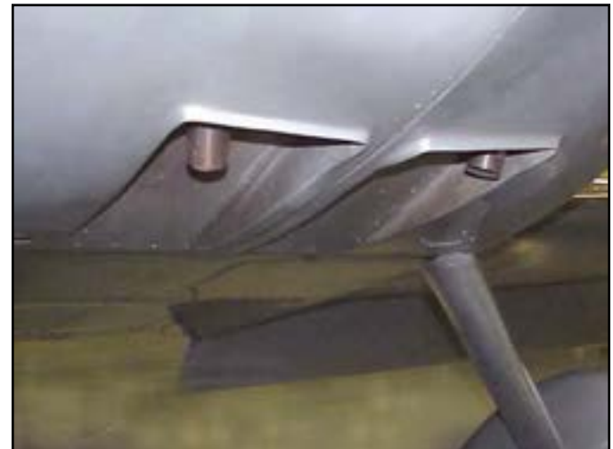
This view of a completed cowl clearly shows the air deflector lips which are added to the front of the exhaust cut-out. These lips create a low pressure area which draws the cooling air through the cowl. These lips are particularly important when the airplane is in a climb attitude.
