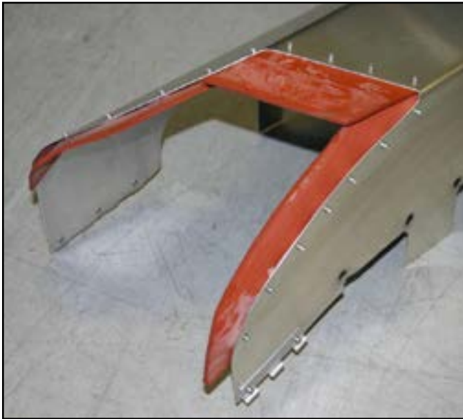
The left cylinder head baffle is shown here with all of the baffle seals installed.
