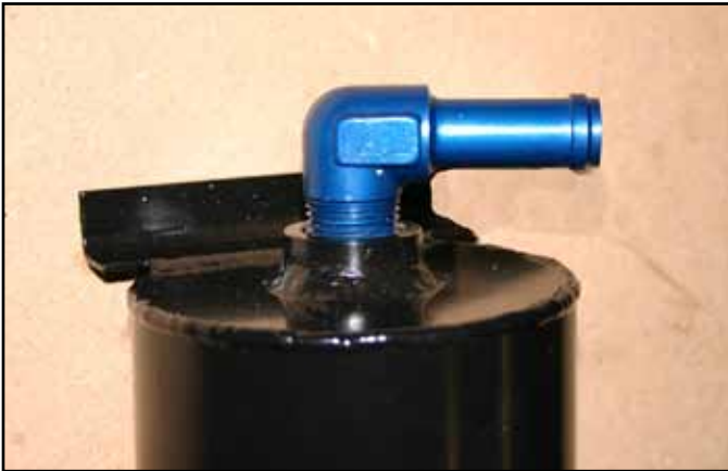
This separator is shown with an AN912 reducer and AN842 hose elbow.
