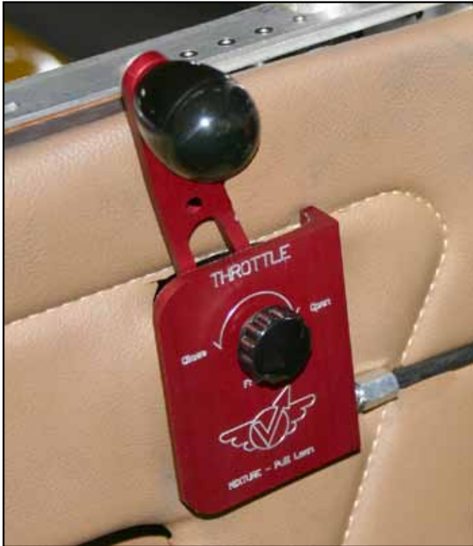
This throttle quadrant has been installed without the mixture control mounting bracket.
