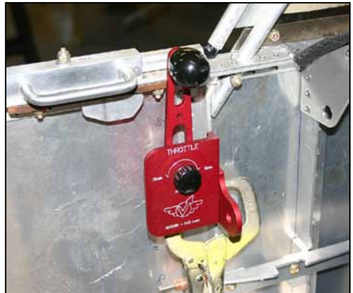
The throttle quadrant is clamped in place prior to drilling the mounting holes. Note that this aircraft needs to have the forward canopy handle moved aft to eliminate interference with the throttle quadrant.
