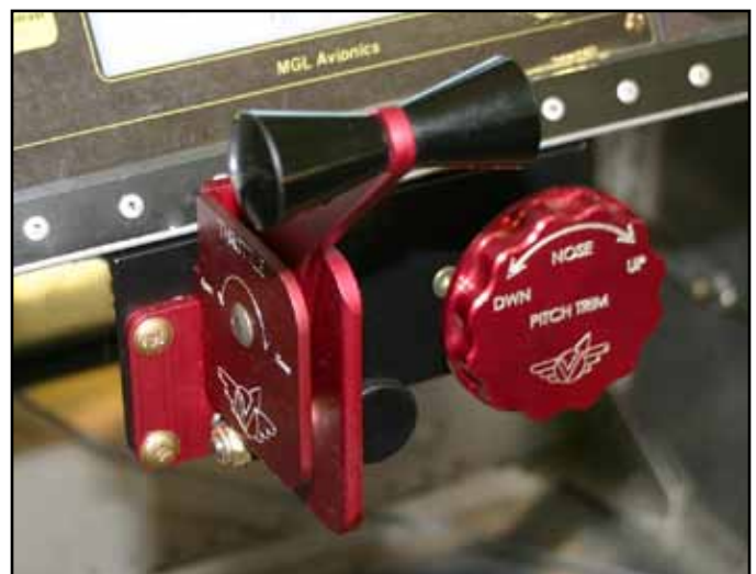
This center-mounted quadrant is attached to a 1/8" thick angle extrusion mounted under the panel.
