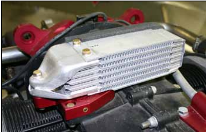
The top-mounted oil cooler positions the oil cooler on top of the case, near the accessory plate.
