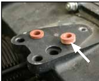
The arrow in this photo shows one of the seals before it is installed in its port.
