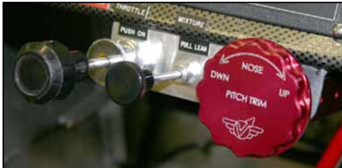
Install the trim cable before installing the trim unit in your airplane.
