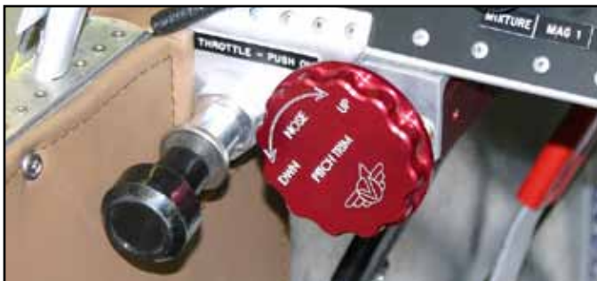
Two mounting locations for the trim unit: Upper photo is in a Sonex ST, lower photo is a standard Sonex. Both aircraft have the trim unit mounted for operation with the "throttle" hand.
